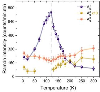
Fig. 3 The Stokes Raman spectral intensities, as a function of temperature, of the  $A_q^1$ ,  $A_q^2$ , and  $A_q^3$  modes. From 125 K down to 70 K, the  $A_q^2$  mode exhibits zero intensity due to complete suppression. The vertical dashed line indicates 120 K.
