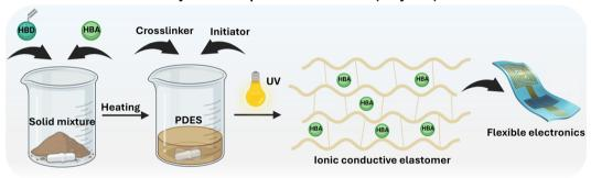
Scheme 2 Examples of chemical structures of hydrogen bond acceptors (HBAs) and donors (HBDs), which have been combined to obtain PDESs (top). Schematic illustration of polyDES preparation by UV-photopolymerization resulting in ionic elastomers for flexible electronics.
