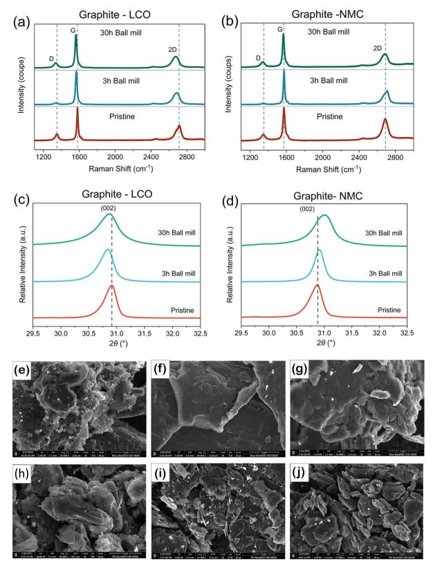
Fig. 2 Comparison of the impact of ball milling on PRG, Raman spectra of (a) PRG-LCO and (b) PRG-NMC, (c) XRD patterns in selected  $2\theta$ regions highlighting the (002) reflection of (d) PRG-LCO and (e) PRG-NMC, microstructures of (e) PRG-LCO, (f) PRG-LCO-3h, and (g) PRG-LCO-30h, and microstructures of (h) PRG-NMC, (i) PRG-NMC-3h, and (j) PRG-NMC-30h.
