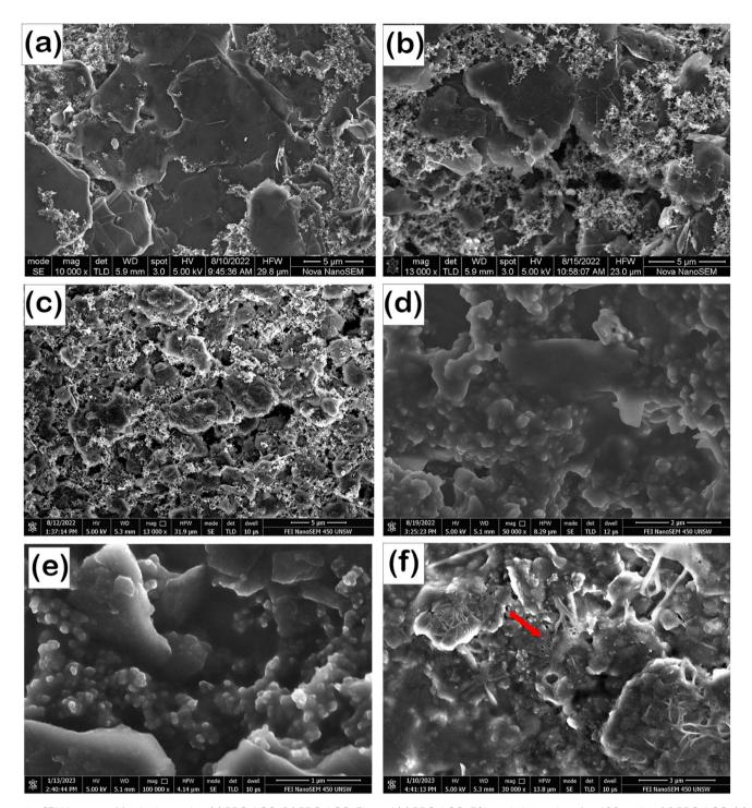
Fig. 5 SEM images of fresh electrodes, (a) PRG-LCO, (b) PRG-LCO-3h, and (c) PRG-LCO-30h and electrodes after 100 cycles, (d) PRG-LCO, (e) PRG-LCO-3h, and (f) PRG-LCO-30h
