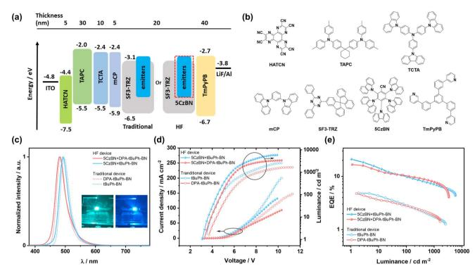
Fig. 7 (a) Schematic of the device stack of the OLEDs; (b) chemical structures of the organic layers; (c) EL spectra recorded at 5 V, the insets are the photograph images of the HF devices for tBuPh-BN (left) and DPA-tBuPh-BN (right); (d) JVL characteristics; (e) EQE vs. luminance for the OLEDs.
