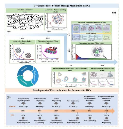
Fig. 4 Timeline of key developments in the sodium storage mechanism (a) and electrochemical performance (b) of HCs.
