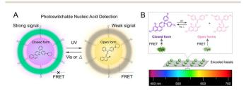
Fig. 7 (A) Photoswitch-mediated FRET-based detection of nucleic acids. The Adapted with permission from ref. 107. Copyright 2021 American Chemical Society. (B) Photoswitch-based fluorescence encoding particles for multiplexed detection. Adapted with permission from ref. 109. Copyright 2022 American Chemical Society.
