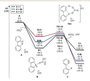
Fig. 10 Calculated energy diagram (in kcal mol<sup>-1</sup>) for the formation of arynes from hypervalent halonium.
