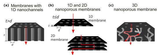
Fig. 2 Illustrations of the solid-state membrane film structures included in our review: (a) 1D nanochannels with a longer channel length (or film thickness, t) than the diameter (d) of the nanopores; (b) 2D membrane thin films with 1D nanopores where d > t or the stacks of such 1D membranes (called 2D membranes); (c) 3D nanoporous membranes with irregularly connected nanopores.
