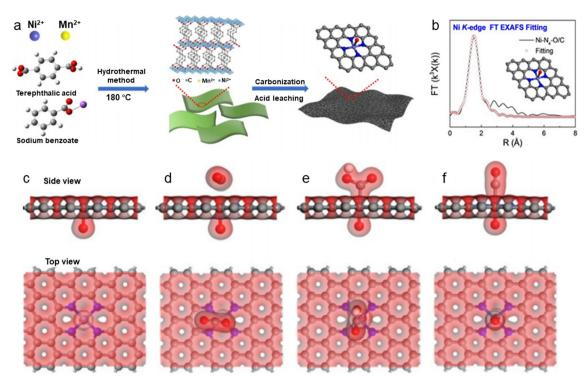
Fig. 10 (a) Illustration of the synthesis process; (b) EXAFS fitting curves in R space. Inset: Corresponding schematic model of Ni-N<sub>4</sub>-O/C; (c)-(f) side view and top view of structural evolution of electrochemical CO<sub>2</sub>RR for Ni-N<sub>4</sub>-O/C (Ni cyan, N blue, O red, H white, C grey). 48 Reprinted with permission from Wiley-VCH, copyright 2020.
