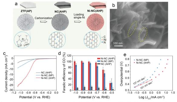
Fig. 5 (a) Schematic illustration of the preparation route for Ni-NC(AHP); (b) FESEM images of Ni-NC(AHP); the dash circles indicate the openings and parallel walls of hollow plates; (c–e) CO<sub>2</sub> electroreduction performance of samples; (c) LSV curves in CO<sub>2</sub>-saturated 0.5 M KHCO<sub>3</sub> solution; (d) comparison of CO faradaic efficiency at various potentials; and (e) Tafel plots towards CO product.<sup>41</sup> Reprinted with permission from Wiley-VCH, copyright 2021.
