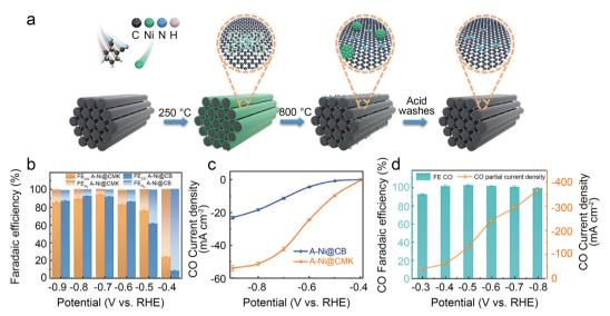
Fig. 4 (a) Schematic illustration of the synthesis of A-Ni@CMK; (b)  $FE_{CO}$  and  $FE_{H_2}$  of A-Ni@CMK and A-Ni@CB in the H-type cell; (c)  $j_{CO}$  of A-Ni@CMK and A-Ni@CB in the H-type cell; and (d) electrocatalytic activity of A-Ni@CMK in the flow cell. 40 Reprinted with permission from Wiley-VCH, copyright 2021.
