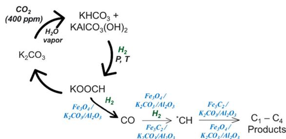
**Scheme 1** Proposed mechanism for the conversion of captured CO<sub>2</sub> to C–C coupled products in the presence of Fe/KA.
