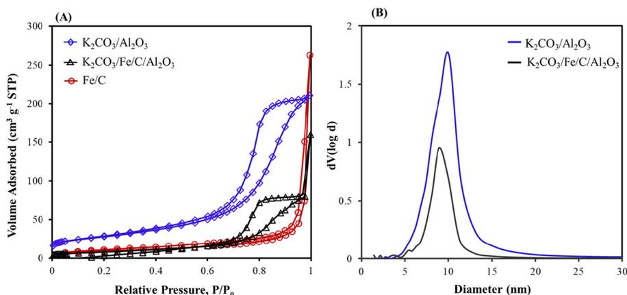
Fig. 3 (A) Nitrogen adsorption–desorption isotherms of K<sub>2</sub>CO<sub>3</sub>/Al<sub>2</sub>O<sub>3</sub>, K<sub>2</sub>CO<sub>3</sub>/Fe/C/Al<sub>2</sub>O<sub>3</sub>, and Fe/C and (B) Barrett–Joyner–Halenda (BJH) curves for K<sub>2</sub>CO<sub>3</sub>/Al<sub>2</sub>O<sub>3</sub>, and K<sub>2</sub>CO<sub>3</sub>/Fe/C/Al<sub>2</sub>O<sub>3</sub>.
