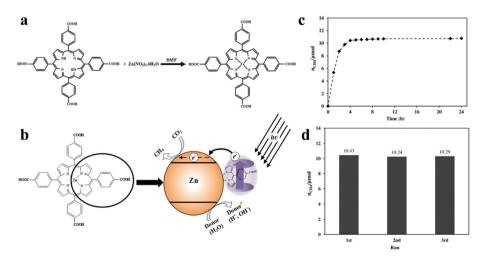
Fig. 9 (a) Synthetic reaction scheme for Zn/PMOF. (b) Mechanism of photocatalytic reduction of CO<sub>2</sub> over Zn/PMOF with H<sub>2</sub>O vapor as a sacrificial agent. (c) The photocatalytic performance of Zn/PMOF under UV/Visible light. (d) Recycling tests for photocatalytic reduction of CO<sub>2</sub> under UV/Visible light over Zn/PMOF. Reproduced from ref. 127. Copyright 2022 Elsevier.
