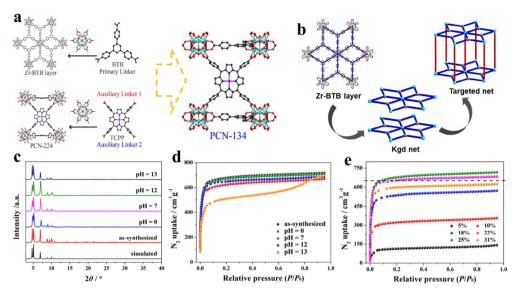
Fig. 6 Design of mixed-linker Zr-MOFs: (a) and (b) PCN-134 and PCN-224 formed by the 6-connected Zr<sub>6</sub> cluster and TCPP. (c) The XRD patterns and (d) the N2 isotherms after immersion in aqueous solutions with different pH values at room temperature for 24 h. (e) Effects of TCPP defects of the PCN-134 system on N<sub>2</sub> uptake measured at 77 K. Reproduced from ref. 98. Copyright 2022 ACS.
