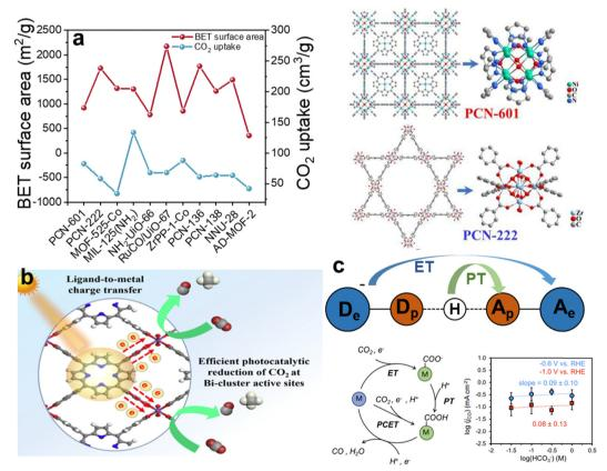
Fig. 8 (a) The BET surface area and the  $CO_2$  uptake of PCN-601 and the structure of PCN-601 and PCN-222. Reproduced from ref. 113. Copyright 2022 ACS. (b) The electron-transfer mechanisms of SC-Bi-PMOFs. Reproduced from ref. 114. Copyright 2022 Elsevier. (c) The mechanisms of ET-PT and PCET and the pattern of  $log(j_{CO})$  vs.  $log(HCO_3^-)$ . Reproduced from ref. 115. Copyright 2022 Wiley.
