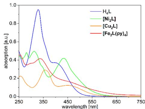
Fig. 3 UV-Vis absorption spectra of  $\text{H}_4\text{L}$ ,  $[\text{Ni}_2\text{L}]$ ,  $[\text{Cu}_2\text{L}]$  and  $[\text{Fe}_2\text{L}(\text{py})_4]$  in DCM ( $c = 1.0 \times 10^{-5}$  M for ligand, Fe and Ni but  $<1.0 \times 10^{-5}$  M for Cu).
