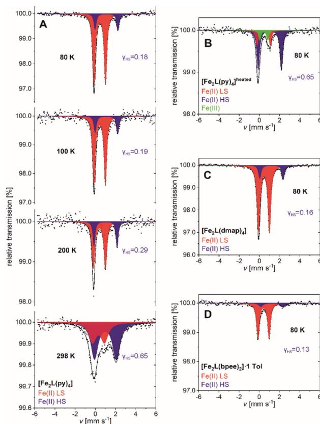
Fig. 8 <sup>57</sup>Fe-Mössbauer spectra of (A)  $[\text{Fe}_2\text{L}(\text{py})_4]$ , (B)  $[\text{Fe}_2\text{L}(\text{py})_4]^{\text{heated}}$ , (C)  $[\text{Fe}_2\text{L}(\text{dmap})_4]$  and (D)  $[\text{Fe}_2\text{L}(\text{bpee})_2] \cdot 1 \text{ Tol}$  recorded at various temperatures.
