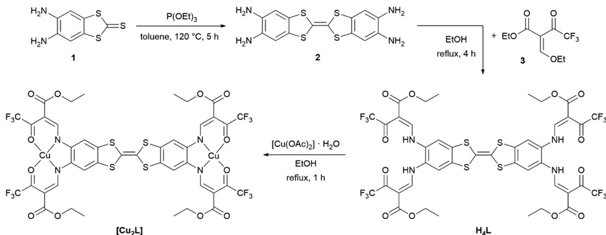
**Scheme 2** Synthesis of the binucleating ligand H<sub>4</sub>L, starting from 4,5-diaminobenzole-1,3-dithiol-2-thione 1 and complex synthesis, exemplified for the copper(II) complex [Cu<sub>2</sub>L].
