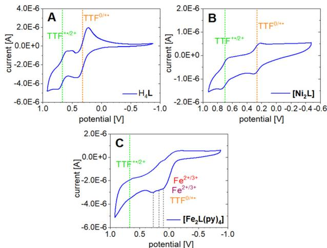
**Fig. 9** Cyclic voltammograms of H<sub>4</sub>L (A), [Ni<sub>2</sub>L] (B) and [Fe<sub>2</sub>L(py)<sub>4</sub>] (C) measured in DCM ( $c = 1.0 \times 10^{-3}$  M) with NBu<sub>4</sub>PF<sub>6</sub> ( $c = 0.1$  M) as electrolyte, on a platinum working and counter electrode with a saturated calomel reference electrode (SCE) and a scan rate of 50 mV s<sup>-1</sup>. Potentials are reported in reference to Fc/Fc<sup>+</sup>.
