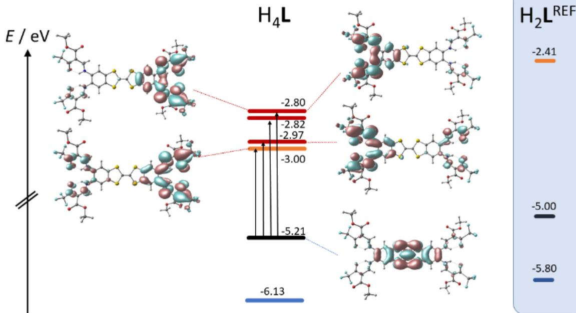
Fig. 4 Kohn–Sham frontier MO energy diagram and orbital plots of the binucleating ligand  $H_4L$ ; vertical arrows denote dominant orbital parentage of Vis-transitions at low energy; for sake of comparison, MO energy levels of a related mononucleating ligand  $H_2L^{REF}$  are re-plotted from ref. 8
