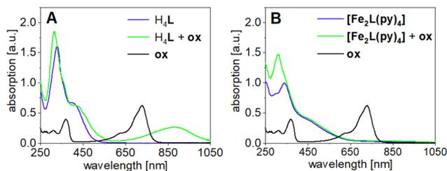
**Fig. 11** UV-Vis absorption spectra of (A) the ligand  $H_4L$  and (B)  $[Fe_2L(py)_4]$  in DCM after addition of one aliquot oxidation agent  $[N(C_6H_5Br_4)_3]^+ [(3,5-(CF_3)_2C_6H_3)_4B]^- ox$ ; ( $c = 2.0 \times 10^{-5}$  M).
