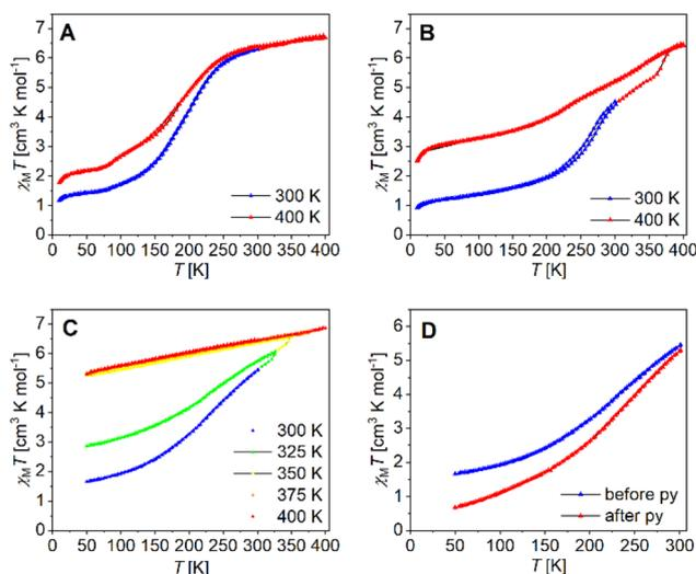
Fig. 7 Temperature dependence of  $\chi_{\text{M}}T$  of (A)  $[\text{Fe}_2\text{L}(\text{dmap})_4]$ , (B)  $[\text{Fe}_2\text{L}(\text{bpee})_2] \cdot 1 \text{ Tol}$ , (C)  $[\text{Fe}_2\text{L}(\text{py})_4]$  in different temperature ranges and (D)  $[\text{Fe}_2\text{L}(\text{py})_4]$  before and after flushing the sample with pyridine saturated argon.
