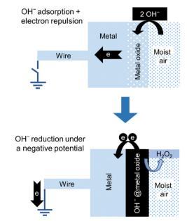
Fig. 15 Stepwise description of the two steps in the negative electrode of a hygroelectric cell: (top) adsorption: an isolated electroneutral acidic oxide surface in contact with moisture adsorbs OH- ions acquiring negative charge. (bottom) Redox reaction: electron transfer from OHions to the electrode produces hydrogen peroxide. Adapted with permission from ref. 131. Copyright 2023. American Chemical Society.
