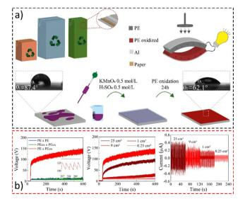
Fig. 20 (a) Fabrication of a simple triboelectric energy harvesting device using a laminated food packaging film. LDPE surface oxidation with  $KMnO_4$  solution lowered the water contact angle. (b) Open-circuit voltage using different dielectric-to-dielectric pairs and the (d) open-circuit voltage and (e) short-circuit current on samples with different sizes. Adapted from ref. 192, Copyright (2023), with permission from Elsevier.
