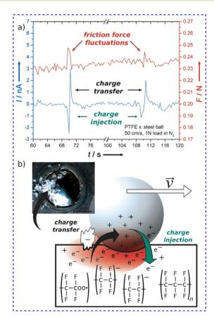
Fig. 18 (a) Friction force fluctuations and tribocurrent at the metal-PTFE interface and (b) the suggested mechanism. Electron injection in PTFE, simultaneous to the mechanochemical homolytic rupture of PTFE bonds produces excess negative charge on PTFE. The attractive force between two surfaces with opposite charges increases the friction force. Reprinted from ref. 178, Copyright (2023), with permission from John Wiley and Sons.
