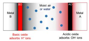
Fig. 14 Electrified compartments in a hygroelectric cell made from parallel plates of conductive materials, metals A and B. The oxide AO adsorbs OH<sup>-</sup> ions becoming negative and repelling negative charge in the supporting metal, while BO becomes positive by adsorbing H<sup>+</sup> ions. Excess charge in the oxides produces a potential difference between metals A and B. Adapted with permission from ref. 131. Copyright 2023. American Chemical Society
