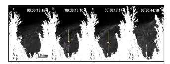
Fig. 10 Video frames from the same area, showing an ice needle formation by a non-classical crystallization<sup>69</sup> mechanism. There is no sign of a needle in frame (a) but it appears faintly in the following frame. Needle contrast and thickening increases from (b)-(d). The time difference between consecutive frames is 0.04 s.
