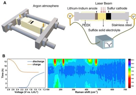
Fig. 15 (A) Schematic of an operando Raman spectroscopic cell for solid-state batteries and the corresponding components of the setup. (B) Timevoltage profile of a solid-state Li-S battery and the corresponding operando Raman spectra contour. Reproduced with permission from ref. 162. Copyright 2023 Wiley-VCH GmbH.
