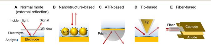
Fig. 4 Different electrochemical vibrational spectroscopic modes. (A) Normal mode (external reflection). (B) Nanostructure-based mode. NP is an abbreviation for nanoparticle. (C) ATR-based mode. (D) Tip-based mode. (E) Fiber-based mode.
