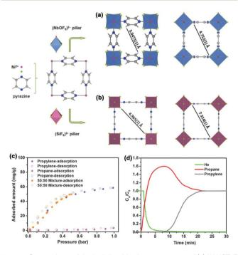
Fig. 11 Comparison of the building block arrangement of (a) KAUST-7 and (b) SIFSIX-3-Ni. (c) Adsorption isotherms of  $C_3H_6$ ,  $C_3H_8$ , and an equimolar mixture of  $C_3H_6/C_3H_8$  on KAUST-7 at 298 K. (d) Breakthrough curves for an equimolar  $C_3H_6/C_3H_8$  mixture on KAUST-7 at 298 K. Reproduced from ref. 64 with permission from copyright 2016, The American Association for the Advancement of Science.
