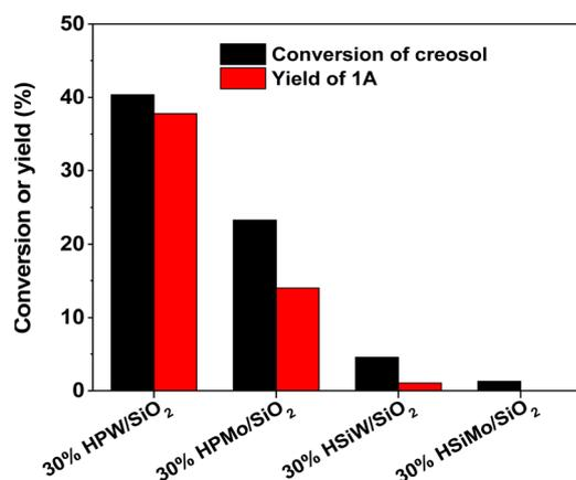
Fig. 1 Creosol conversions and the yields of **1A** over the different heteropolyacid catalysts. Reaction conditions: 333 K, 2 h; 25 mmol creosol, 10 mmol formaldehyde, and 0.1 g catalyst were used in each test.
