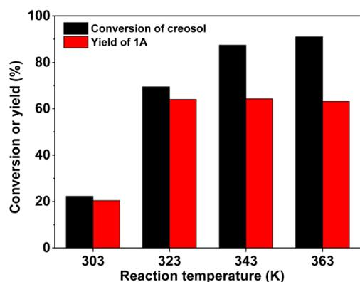
Fig. 5 Creosol conversion and the yield of **1A** over the 40% HPW/SiO<sub>2</sub> catalyst as a function of the reaction temperature. Reaction conditions: 6 h; 20 mmol creosol, 10 mmol formaldehyde, and 0.15 g catalyst were used in each test.
