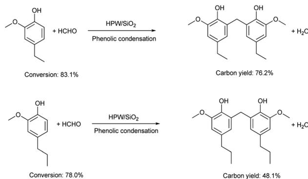
Fig. 6 Conversions of lignin-derived phenols and the carbon yields of different bisphenols over the 40% HPW/SiO<sub>2</sub> catalyst. Reaction conditions: 373 K, 6 h; 20 mmol phenol, 10 mmol formaldehyde and 0.15 g 40% HPW/SiO<sub>2</sub> catalyst were used in the test.
