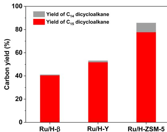
Fig. 7 Yields of different dicycloalkanes from the HDO of **1A** over the Ru-based catalyst. Reaction conditions: 473 K, 4 MPa H<sub>2</sub>, 5 h; 0.2 g **1A**, 0.1 g catalyst; 40 mL solvent was used for each test.
