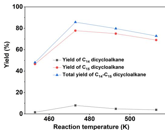
Fig. 9 Yields of different dicycloalkanes from the HDO of **1A** over the Ru/H-ZSM-5 catalyst as a function of the reaction temperature. Reaction conditions: 4 MPa  $\text{H}_2$ , 5 h; 0.2 g **1A**, 0.1 g catalyst; 40 mL cyclohexane (used as solvent) was used for each test.
