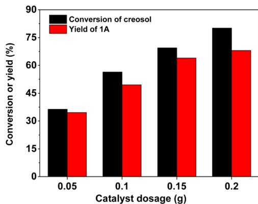
Fig. 4 Creosol conversions and the yields of **1A** over the 40% HPW/SiO<sub>2</sub> catalyst as a function of the catalyst dosage. Reaction conditions: 323 K, 6 h; 20 mmol creosol and 10 mmol formaldehyde were used in each test.
