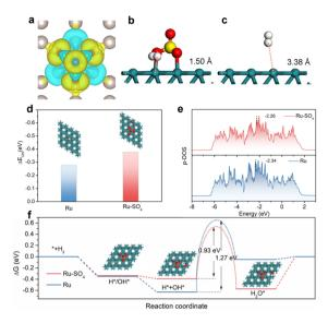
Fig. 4 (a) Calculated differential charge density for  $Ru-SO_4$ . The blue and yellow areas correspond to the depletion and accumulation of electrons, respectively. The optimal theoretical structure of  $H_2$  on  $Ru-SO_4$  (b) and Ru (c). (d) The adsorption energy of  $OH^*$  on  $Ru-SO_4$  and Ru with the corresponding optimal theoretical structure. The projected density of states (e) and the reaction pathways (f) of Ru and  $Ru-SO_4$ .
