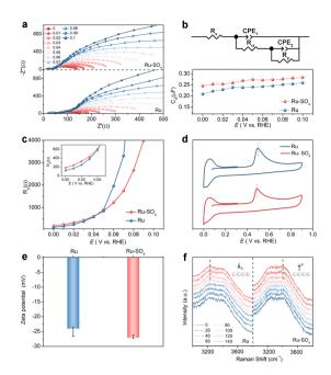
Fig. 3 (a) Nyquist plots of Ru and Ru-SO<sub>4</sub> in the potential range from 0 V to 0.1 V. (b) The equivalent circuit and the  $C_{\rm cl}$  at different potentials for Ru and Ru-SO<sub>4</sub>. (c) The  $R_{\rm p}$  at different potentials for Ru and Ru-SO<sub>4</sub>. (d) CO stripping curves in CO-statured 0.1 M KOH. (e) Zeta potentials of Ru and Ru-SO<sub>4</sub>. (f) *In situ* Raman spectra of interfacial water on Ru and Ru-SO<sub>4</sub> in 0.1 M KOH at 0 mV to 140 mV.
