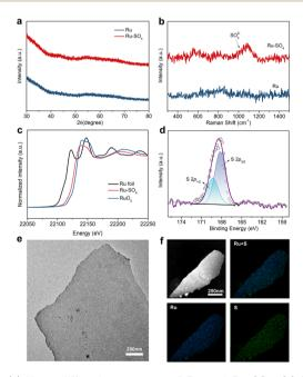
Fig. 1 (a) X-ray diffraction patterns of Ru and Ru-SO<sub>4</sub>. (b) Raman spectra of Ru and Ru-SO<sub>4</sub>. (c) Ru K-edge XANES of Ru foil, Ru-SO<sub>4</sub> and RuO<sub>2</sub>. (d) XPS spectra of S 2p for Ru-SO<sub>4</sub>. (e) Typical TEM image and (f) EDX mapping images for Ru-SO<sub>4</sub>.
