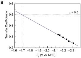
Fig. 2 (A) Cyclic voltammogram of disulfide 1. Electrolyte is anhydrous acetonitrile solution containing 1.5 mM RSSR and 0.1 M tetrabutylammonium hexafluorophosphate. (B) Peak potential  $(E_p)$ -transfer coefficient ( $\alpha$ ) plot of disulfide 1.
