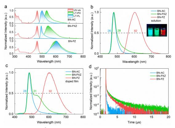
Fig. 4 (a) UV-vis absorption (Abs., in  $1 \times 10^{-5}$  M toluene), steady-state fluorescence (LT-FL, 77 K in neat films), and phosphorescence (LT-Ph, 77 K in neat films) spectra. (b) Photoluminescence spectra in toluene ( $1 \times 10^{-5}$  M). (c) Photoluminescence spectra in 15 wt% doped films (host: mCBP). (d) Transient photoluminescence decay profiles (doped films in vacuo).
