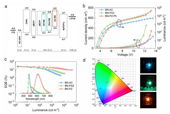
Fig. 5 (a) Device structure and energy level diagram of the materials used. (b) Current density and luminance versus voltage (J-V-L). (c) External quantum efficiency versus luminance (EQE-L) curves of the devices (inset: EL spectra of the devices). (d) The color coordinates of the devices on the CIE 1931 color space and the photographs showing the emission color of the 15 wt%-doping devices
