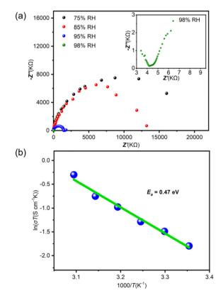
(a) Nyquist plots of the pelleted sample of T3-MEP at different RH at 25 °C. (b) Arrhenius plots of proton conductivity vs. the temperature for T3-MEP under 98% RH.
