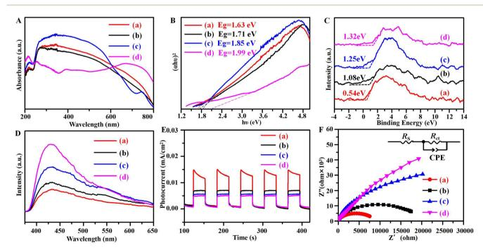
Fig. 6 (A) UV-vis DRS spectra, (B) Tauc plots, (C) VB-XPS spectra, (D) PL spectra, (E) transient photocurrent curves, and (F) Nyquist plots for EIS for the prepared samples. ((a) re-CuNiFe-MMOs, (b) re-CuFe-MMOs, (c) re-CuNi-MMOs, (d) re-FeNi-MMOs).
