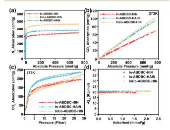
Fig. 3 (a) N<sub>2</sub> adsorption and desorption isotherms at 77 K, (b) lowpressure CO<sub>2</sub> adsorption isotherms at 273 K and (c) high-pressure CO<sub>2</sub> adsorption isotherms at 273 K for In-ABDBC-HIN, InCo-ABDBC-HIN, and In-ABDBC-HAIN. (d) Isosteric heat of adsorption (Qst).
