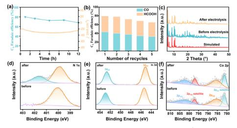
Fig. 5 (a) Long-term durability of InCo-ABDBC-HIN. (b) FE after five times electrolysis at -2.2 V vs. Ag/Ag<sup>+</sup>. (c) Comparison of XRD spectra, (d) N 1s, (e) In 3d and (f) Co 2p XPS of InCo-ABDBC-HIN before and after electrolysis.
