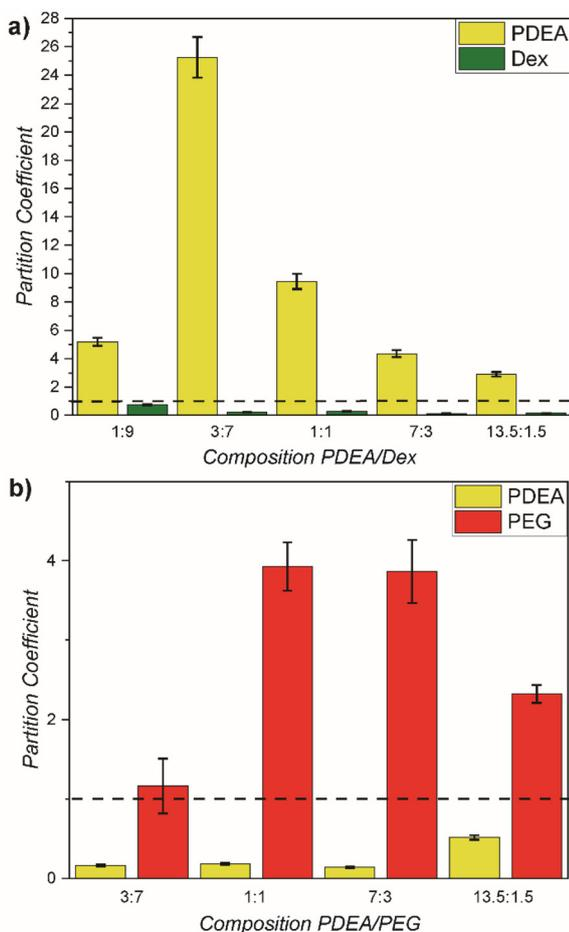
**Fig. 2** Partitioning of polymers in ATPS (values above 1, *i.e.* the dotted line, mean enrichment in top phase; values below 1 mean enrichment in bottom phase): (a) partitioning of PDEA<sub>55k</sub> and Dex in ATPS of various and (b) partitioning of PDEA<sub>55k</sub> and PEG in ATPS of various composition.
