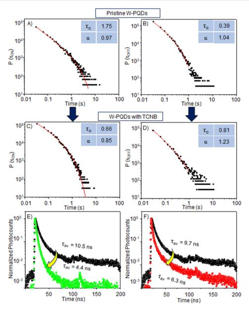
Fig. 4 Blinking time distributions for >400 single PQDs. Probability distributions of (A, C) ON- and (B, D) OFF-times for W-PQDs (A, B) without or (C, D) with TCNB. (E and F) W-PQD's PL decays with or without (E) TCNB and (F) TCNQ. The quencher concentration is 10 µM in both cases.
