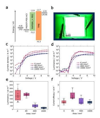
Fig. 3 (a) Usage of a TPBi electron transport layer improves devices performance and enables (b) homogeneous emission from a 1600 mm<sup>2</sup> PeLED. Current density-voltage (c) and luminance-voltage (d) characteristics show greatly improved performance of champion devices. The luminance distribution (e) and current efficacy distribution (f) for all fabricated devices.
