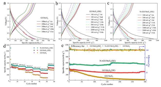
Fig. 4 (a-c) are charge/discharge profiles at the different current densities, (d) rate performance, and (e) cycling performance at 200 mA g<sup>-1</sup> of GO/ MoS<sub>2</sub>, GO/MoS<sub>2</sub> (ISE) and N-rGO/MoS<sub>2</sub> (ISE)
