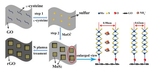
Scheme 1 Schematic illustration of the synthesis of N-rGO/MoS<sub>2</sub>(ISE).
