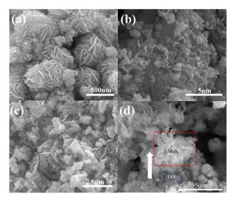
Fig. 2 SEM images of (a) GO/MoS<sub>2</sub>, (b) GO/MoS<sub>2</sub> (ISE) and (c and d) NrGO/MoS<sub>2</sub> (ISE).
