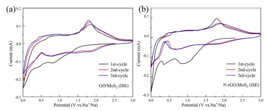
Fig. 5 CV curves at a scanning rate of 0.2 mV s<sup>-1</sup> of (a) GO/MoS<sub>2</sub> (ISE) and (b) N-rGO/MoS<sub>2</sub> (ISE).
