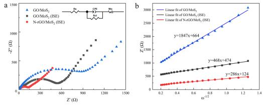
Fig. 6 (a) EIS spectra of GO/MoS<sub>2</sub> (ISE) and N-rGO/MoS<sub>2</sub> (ISE) (inset is equivalent circuit); (b) the linear fits of Z' and  $\omega^{-1/2}$  of GO/MoS<sub>2</sub> (ISE) and N-rGO/MoS<sub>2</sub> (ISE) and MoS<sub>2</sub> (ISE).
