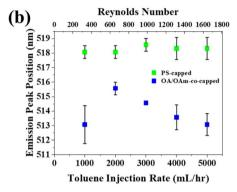
Fig. 2 (a) Effect of  $\Omega_{toluene}$  on PLQY and (b) emission peak position of PS-capped CsPbBr $_3$  PNCs via capitalizing on star-like PAA-b-PS as nanoreactor and OA/OAm-co-capped CsPbBr $_3$  PNCs (control sample).
