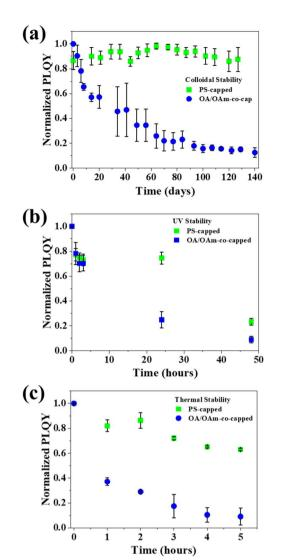
Fig. 5 (a) Colloidal, (b) UV, and (c) thermal (at 80 °C) stabilities of PS-capped and OA/OAm-co-capped CsPbBr $_3$  PNCs (control sample) synthesized at optimized conditions ( $Q_{tol} = 5000$  mL h $^{-1}$  and  $Q_{precursor} = 60$  mL h $^{-1}$ ).
