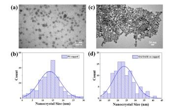
Fig. 4 TEM image and size distribution of (a and b) PS-capped CsPbBr $_3$  PNCs and (c and d) OA/OAm-co-capped CsPbBr $_3$  PNCs (control sample). Both samples were synthesized at optimized conditions ( $Q_{tol} = 5000 \text{ mL h}^{-1}$  and  $Q_{precursor} = 60 \text{ mL h}^{-1}$ ).
