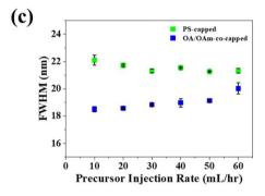
Fig. 3 Effect of  $Q_{\rm precursor}$  on (a) PLQY, (b) emission peak position, and (c) FWHM of PS-capped CsPbBr<sub>3</sub> PNCs and OA/OAm-co-capped CsPbBr<sub>3</sub> PNCs (control sample), where  $Q_{\rm tol}$  was held constant at the optimized 5000 mL h<sup>-1</sup>.
