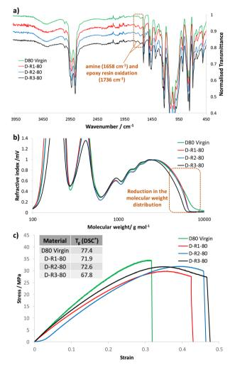
Fig. 13 Characterisation of dioxazaborocane D80 before mechanical recycling (virgin), and after one (D-R1-80), two (D-R2-80) and three (D-R3-80) recycling processes (at 170 °C) by (a) Infrared spectroscopy, (b) GPC after chemical recycling in THF/pinacol and (c) tensile testing with  $T_{\rm q}$  by DSC (inset, \*run at 100 °C min<sup>-1</sup>).
