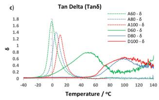
Fig. 5 DMTA analysis of D60-D100 and A60-A100 materials. (a) overlay of storage modulus curves (E'), (b) overlay of loss modulus curves (E'') and (c) overlay of  $\tan \delta$  curves (E''/E').
