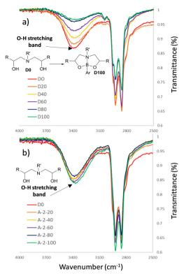
Fig. 6 FTIR overlays of (a) epoxy-amine-dioxazaborocane materials (D0-D100, inset: representative molecular structure of D0 and D100) and (b) epoxy-amine thermoset materials (A<sup>2</sup>20-A<sup>2</sup>100, inset: representative molecular structure)
