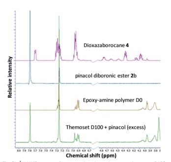
Fig. 8 <sup>1</sup>H-NMR spectra of epoxy-amine-dioxazaborocane thermoset D100 after chemical recycling via pinacol methodology (according to Fig. 7b).
