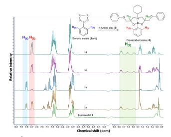
Fig. 1 <sup>1</sup>H-NMR analysis of the reaction mixtures of boronic esters **1a-d** with model β-amino diol 3. Hydrogen environments of interest are indicated as according to the colours H-atom (H1, H2 and H3) labelled on both the molecule structures and spectra.
