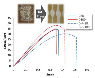
Fig. 12 Stress over strain curves for D80/D<sup>R</sup>80 and D100/D<sup>R</sup>100 (pre and post mechanical recycling). Inset: Image of D100 before and after mechanical recycling, by hot press and laser cutting into dog bones for tensile testing
