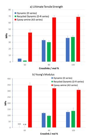
Fig. 11 (a) Ultimate tensile strength and (b) Young's modulus, data for D60-D100 and A<sup>3</sup>60-A<sup>3</sup>100 materials.
