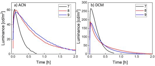
Fig. 5 Time-dependence of the luminance [cd m $^{-2}$ ] of LECs ITO/PEDOT:PSS/iTMC:IL(4:1)/Al, (iTMC: **7** (black), **8** (red) and **9** (blue)) with the active layer prepared from solutions in ACN (a) and DCM (b). All the devices shown were driven with a pulsed current with an average current density of 50 A m $^{-2}$ .
