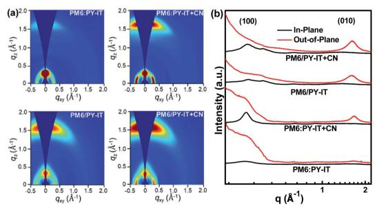
Fig. 4 (a) The 2D-GIWAXS patterns of PM6:PY-IT, PM6:PY-IT + CN, PM6/PY-IT and PM6/PY-IT + CN films. (b) The in-plane (IP, black line) and out-of-plane (OOP, red line) profiles abstracted from the 2D-GIWAXS patterns of the corresponding films.
