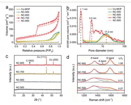
Fig. 3 (a) Nitrogen adsorption/desorption isotherms and (b) DFT pore size distribution curves of Co-MOF and NC-x. (c) XRD and (d) Raman spectra of NC-x.
