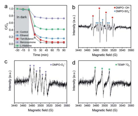
Fig. 11 (a) The effect of radical scavengers on the CR degradation efficiency: [ethanol] = [tert-butanol] = 0.4 M and [benzoquinone] = [Lhistidine] = 0.01 M. (b-d) EPR spectra with the addition of DMPO or TEMP. Reaction condition: [PMS] = 0.15 g  $L^{-1}$  (0.4 mM), catalyst = 0.4 g  $L^{-1}$ , [DMPO] = 0.4 M, and [TEMP] = 0.3 M.
