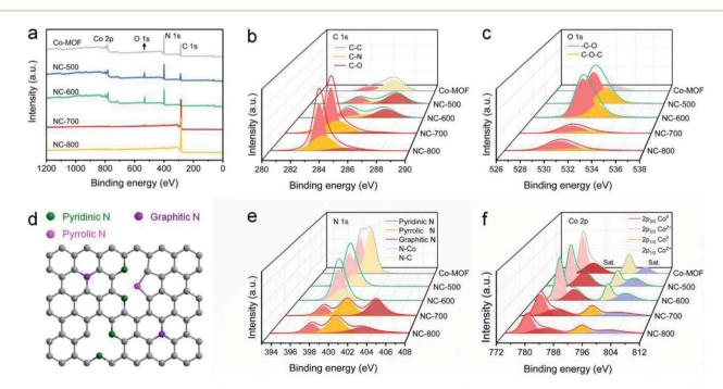
Fig. 4 XPS spectra of Co-MOF and NC-x: (a) full spectra, (b) C 1s spectra, (c) O 1s spectra, (d) scheme of N species, (e) N 1s spectra, and (f) Co 2p spectra.
