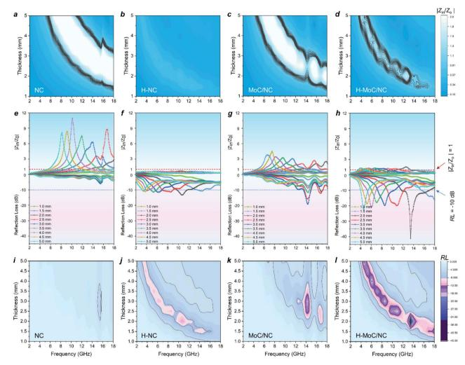
Fig. 4 (a-d) 2D contour map of  $|Z_{in}/Z_0|$  for NC, H-NC, MoC/NC and H-MoC/NC. (e-h) The  $|Z_{in}/Z_0|$  and RL plots of NC, H-NC, MoC/NC and H-MoC/NC. MoC/NC. (i-I) 2D contour map of RL for NC, H-NC, MoC/NC and H-MoC/NC
