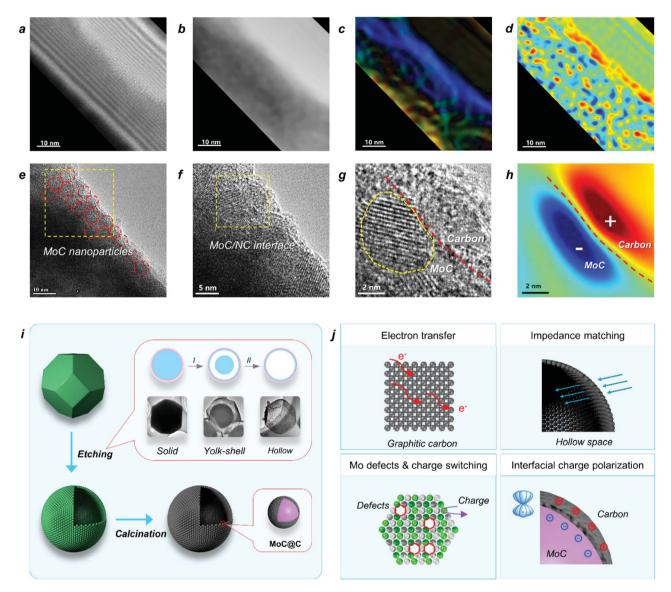
Fig. 5 (a) Hologram. (b) Reconstructed phase image. (c) Electric-filed map. (d) Charge density map. (e) HR-TEM images. (f and g) MoC/NC hetero-interface. (h) Charge distribution on the MoC(–)/carbon(+) interface. (i) Two-step synthetic route and chemical etching mechanism (insert). (j) Illustration schemes of four electromagnetic wave attenuation mechanism.
