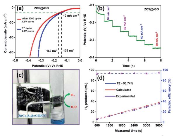
Fig. 6 HER durability test. (a) LSV curve of ZCS@rGO catalyst for before and after 1000 cyclic voltammograms at 100 mV s<sup>-1</sup>in 1.0 M KOH. (b) Multi-step chronopotentiometry curve at 10-80 mA cm<sup>-2</sup>, (c) digital photograph display of H<sub>2</sub> gas evolution, and (d) faradaic efficiency of HER by using ZCS@rGO/CC.
