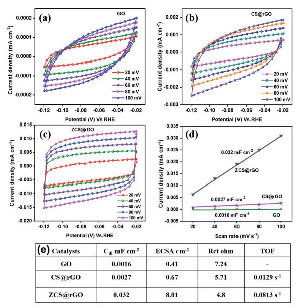
Fig. 5 CV curves with different scan rates from 20–100 mV s<sup>-1</sup> (a) GO/CC, (b) CS@rGO/CC, and (c) ZCS@rGO/CC. (d) Double-layer capacitance measurements (scan rate from 20 to 100 mV  $s^{-1}$ ) of ZCS@rGO, CS@rGO, and GO. (e) The comparative table for electrochemical properties of ZCS@rGO, CS@rGO, and GO.
