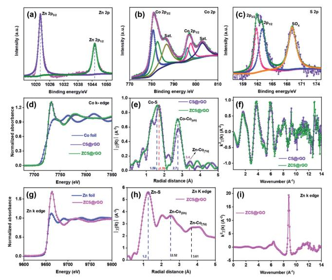
Fig. 3 The XPS analysis of (a) Zn 2p, (b) Co 2p, (c) S 2p spectra of ZCS@rGO catalyst. The XAS analysis, (d) XANES spectra of Co K-edge for CS@rGO, and ZCS@rGO, (e) EXAFS spectra of Co K-edge for CS@rGO, and ZCS@rGO catalysts, (f) EXAFS oscillations of Co K-edge for CS@rGO, and ZCS@rGO catalysts. (q) XANES spectra for Zn K-edge of Zn-foil and ZCS@rGO catalyst. (h) EXAFS spectrum, and (i) EXAFS oscillations for Zn K-edge of ZCS@rGO catalyst, respectively.
