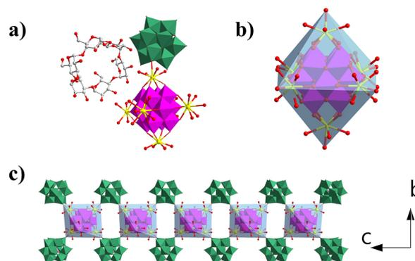
**Fig. 1** (a) The basic building units of **1** with H atoms removed for clarity, (b) octahedral structure of  $\{\text{MnV}_{12}\text{Ce}_6\}$ , (c) 1D IBBs formed by  $\{\text{MnV}_{12}\text{Ce}_6\}$  and  $\{\text{PW}_{10}\text{V}_2\}$ . Colour codes: Mn blue polyhedron, V purple polyhedron, W green polyhedron, Ce yellow ball, O red ball, C grey ball.
