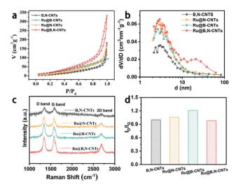
Fig. 3 (a) The  $N_2$  sorption isotherms, (b) the corresponding pore size distributions, (c) the Raman spectra, and (d) the corresponding  $I_D/I_G$ ratios, of the B,N-CNTs, Ru@B,-CNTs, Ru@N-CNTs and Ru@B,N-CNTs.
