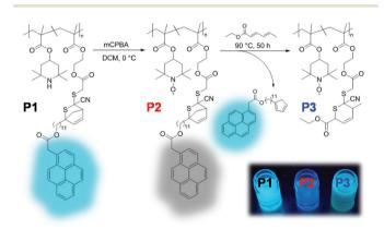
Scheme 5 Synthetic strategy for preparation of a thermally triggered, self-reporting release system. Fluorescence restoration can be seen with the naked eye upon excitation by ultraviolet light (344 nm). Figure reproduced with permission from ref. 48. Copyright, Royal Society of Chemistry, 2017.
