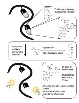
The concept of a polymeric profluorescent system that combines stable nitroxide radicals and doxorubicin and can effectively bind, release and report cancer therapeutics in fluorescence experiments. Figure reproduced with permission from ref. 51. Copyright, Royal Society of Chemistry, 2018.
