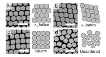
Fig. 8 The (a)  $\Lambda_0$ -lattice, (b)  $\Lambda_1$ -lattice (c) square lattice, and (d) disordered assembly patterns observed in SEM micrographs. Scale bars represent 2 µm. Reproduced with permission from ref. 95. Copyright 2019 American Chemical Society.
