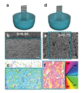
Fig. 7 Assembly in the (a) convective and (d) Landau-Levich regimes, where the (b and e) degree of disorder between assembled helices varies. (c and f) The order parameter, S, was obtained by treating the images to determine the orientation of the helices relative to the withdrawal direction. Scale bars represent 1 µm. Reproduced with permission from ref. 102. Copyright 2020 American Chemical Society.
