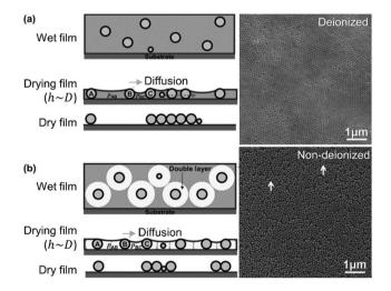
Fig. 6 Particle monolayers prepared using silica particles in (a) non-deionized and (b) deionized water show differing degrees of order as a function of polydispersity. Figure adapted with permission from ref. 164. Copyright 2014 John Wiley & Sons.
