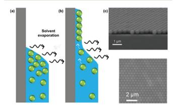
Fig. 4 (a) A high contact angle, where particles are not pinned to the surface and no film deposition is achieved. (b) A good wetting with a contact angle of less than 20°, where convective flux brings particles to the drying line. (c) A continuous monolayer of polystyrene latexes. (c) Reproduced with permission from ref. 101. Copyright 2007 American Chemical Society.
