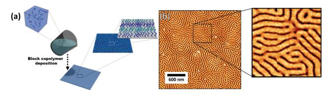
Fig. 12 (a) Block copolymer deposition and self-assembly on a substrate. (b) AFM of a deposited block copolymer (PS(102k)-b-P2VP(97k)) on a silicon substrate. Random organization of domains having constant width.
