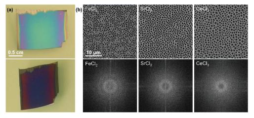
Fig. 19 (a) Photographs of a microperforated film at two different angles. (b) SEM micrographs of macroperforations made by using different salts and their fast Fourier transforms showing differences in the degree of order and the distance between perforations. The scale is the same for all micrographs. Figure adapted with permission from ref. 232. Copyright 2014 John Wiley & Sons.
