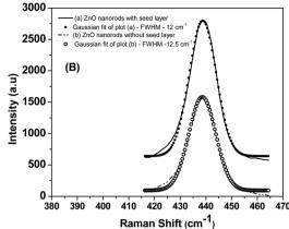
Fig. 4 (A) Raman spectra of (a) ZnO nanorods grown on the Si substrate with a seed layer and (b) ZnO nanorods grown on a Si substrate without a seed layer. (B) The Gaussian fits shown for both the samples at 416 to 464 cm $^{-1}$  reveal the nearly symmetric nature of the E<sub>2</sub> (high) phonon peak at 438 cm $^{-1}$  and the slight asymmetry is seen only at low frequencies.
