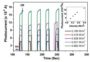
Fig. 8 A plot of photocurrent generated as a function of time upon exposure of the ZnO nanorod film to an Omnicure S 1000 UV-light source (320-500 nm). The ON and the OFF states in the plot show the potential application in UV detection. The inset in the figure shows the peak photocurrent as a function of incident intensity.
