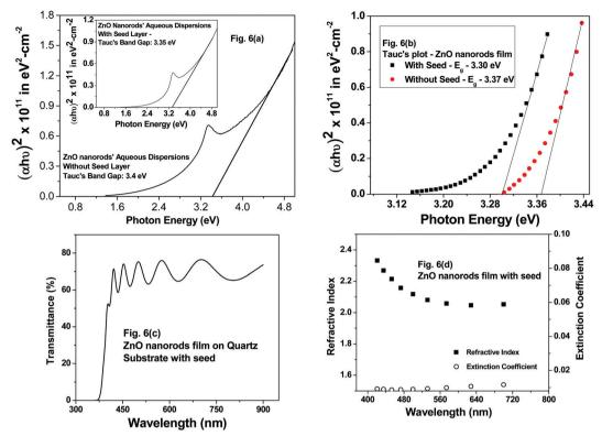
Fig. 6 Tauc's plots to estimate the band gap of ZnO nanorods with and without seed nanoparticles in (a) aqueous dispersions and (b) ZnO nanorod films. (c) Transmittance spectrum and (d) optical constants of ZnO nanorod films with seed ZnO nanoparticles.
