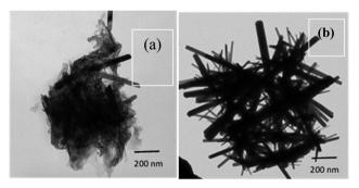
Fig. 2 Bright field images of ZnO nanorods recorded using a 120 kV transmission electron microscope. (a) Observation of floccules, along with the emergence of a few ZnO nanorods. (b) Fully grown ZnO nanorods after the completion of solvothermal treatment under refluxing for 16 hours at 90 °C
