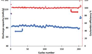
Fig. 7 Long term cycling (blue) and coulombic efficiency (red) of (a) NMO and (b) NMCO for 200 cycles at C/2 (after a pre-conditioning for 5 cycles
