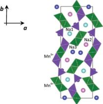
Fig. 1 The crystal structure of  $Na_{0.44}MnO_2$ , showing the ordering of  $Mn^{3+}$ (violet) and Mn<sup>4+</sup> (green) ions and the presence of three distinct crystallographic sites for Na (Na1 cyan, Na2 pink, and Na3 blue).
