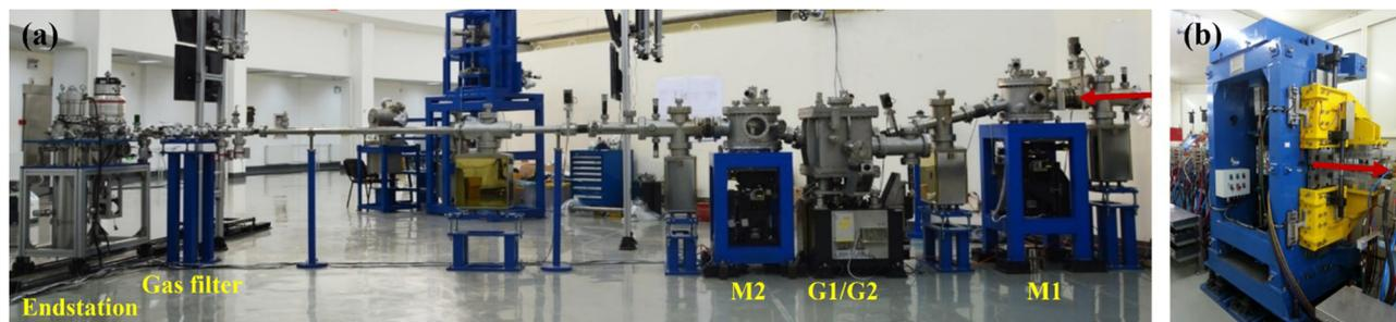
Fig. 1 Photograph of the BL03U beamline<sup>24</sup> (a) and the undulator on the storage ring (b) at Hefei Light Source II. The red arrows denote the direction of light. Adapted and reproduced with permission from the China Academic Journal Electronic Publishing House.
