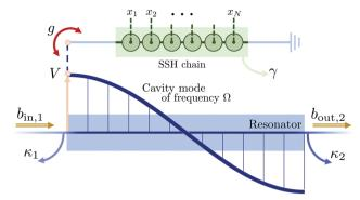
Fig. 1 Schematic picture of a dimerized chain interacting with the photons in a cavity, of frequency  $\Omega$ . The cavity is connected to the input and output ports l = 1, 2 with factors  $\kappa_i$  (i = 1, 2). Fermions and photons interact with coupling strength q, while  $\gamma$  represents the spectral broadening of the fermionic system.
