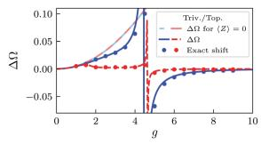
Fig. 4 Plot of  $\Delta\Omega$  (egn (18)) vs. g for both the trivial (blue) and topological (red) phase. The comparison with  $\Delta\Omega$  calculated with  $\langle Z \rangle$  has been included in lighter colors. The dots corresponds to the exact shift (eqn (10)). Parameters:  $\Omega$  = 10,  $\delta$  =  $\pm$ 0.6, N = 20,  $n_{\text{max}}$  = 60.
