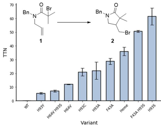
Fig. 2 ATRC activity of myoglobin mutants for the production of  $\gamma$ -lactam **2**. Reaction conditions: 30 mM **1**, 0.1 mol% catalyst, 5 eq. sodium ascorbate, 40 °C, 16 h, PBS-Br (10 mM sodium phosphates, 100 mM NaBr, pH 7.4, 50 mM sodium phosphate/250 mM NaCl for reaction with heme), 3 vol% DMSO, inert atmosphere. TTN – total turnover numbers, average from 2 repetitions.
