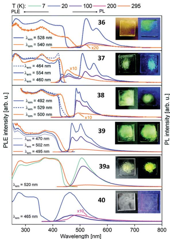
Fig. 11 Solid state excitation and emission spectra of di- and trinuclear PNNP ( $L^{13}$ ) metal complexes **36–40**. PL was excited at  $\lambda_{exc} = 350$  nm for **36–39a** and  $\lambda_{exc} = 330$  nm for **40**.<sup>58</sup>
