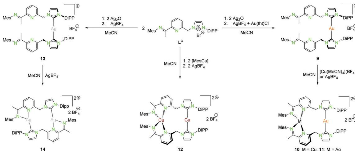
Scheme 4 Synthesis of mononuclear (**9**, **13**), as well as homo- (**12**, **14**) and heterobimetallic (**10**, **11**) NHC<sup>impy</sup> (L<sup>3</sup>) compounds.<sup>43</sup>
