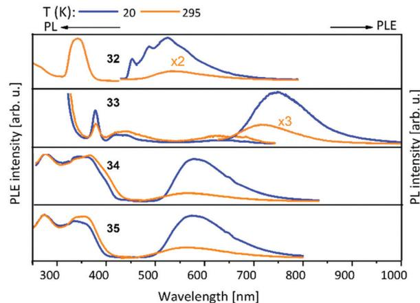
Fig. 10 Solid state excitation and emission spectra of PN<sub>4</sub> (**L**<sup>12</sup>) metal complexes **32**–**35**. PL was excited at  $\lambda_{\text{exc}} = 350$  nm and PLE spectra recorded at  $\lambda_{\text{em}} = 560$  nm for **32**, **33**, **35** and  $\lambda_{\text{em}} = 580$  nm for **34**.<sup>48</sup>
