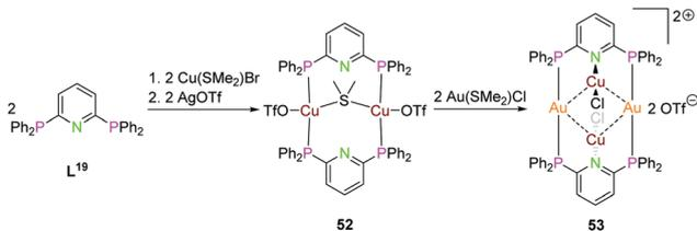
Scheme 14 Synthesis of homo- (**52**) and heterometallic (**53**) compounds with ligand **L**<sup>19</sup>.<sup>18</sup>
