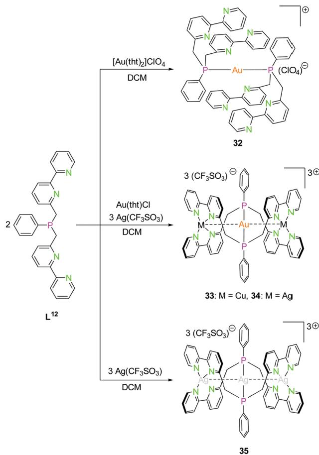
Scheme 10 Synthesis of mononuclear gold(i) (**32**) and trinuclear hetero- (**33**, **34**) and homometallic silver(i) (**35**) PN<sub>4</sub> ( $L^{12}$ ) compounds.<sup>48</sup>
