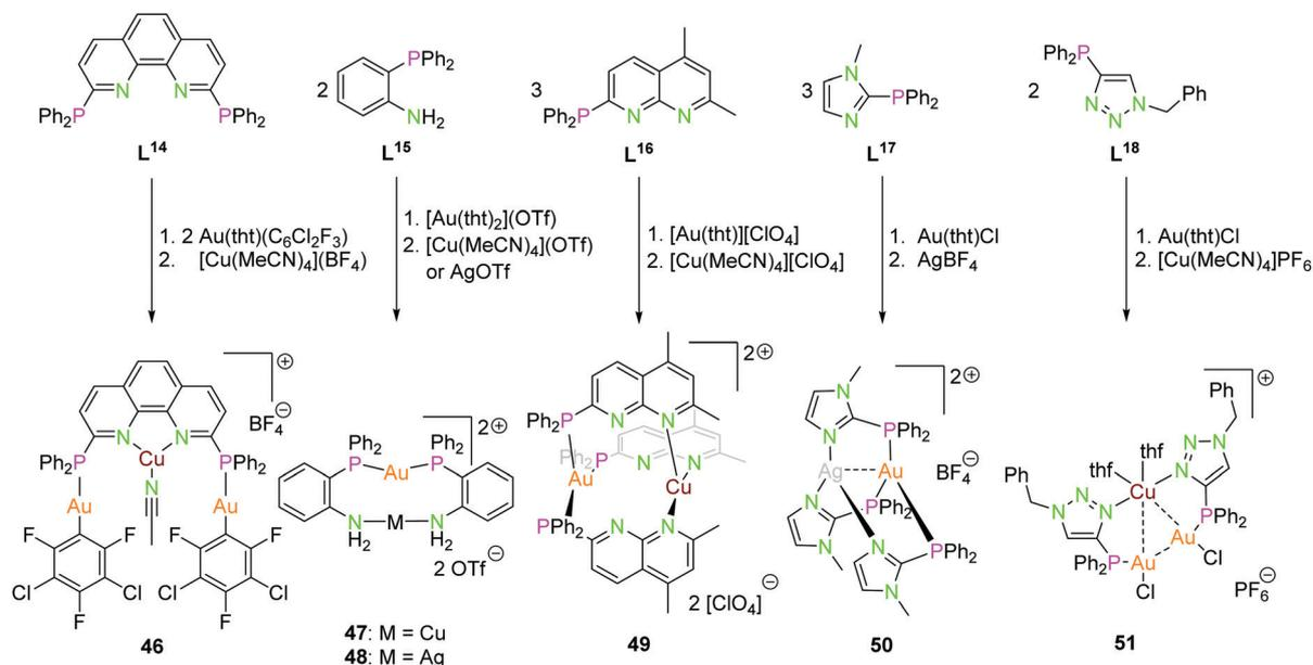
Scheme 13 Synthesis of heterometallic di- (**47**–**50**) and trinuclear (**46**, **51**) compounds with ligands **L**<sup>14</sup>–**L**<sup>18</sup>.<sup>34,50,54,74,75</sup>
