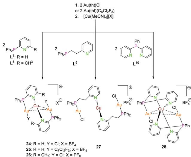
Scheme 8 Synthesis of trinuclear heterometallic PPy ( $L^7$ – $L^{10}$ ) compounds 24–28.<sup>13,51,54</sup>
