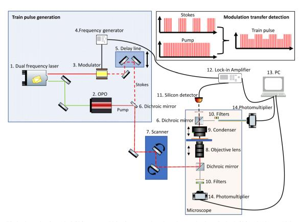
Fig. 3 Simplified schematic of a typical CRS system, which often comprises detection mechanisms for both SRS and other multiphoton imaging modalities.
