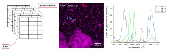
Fig. 8 Hyperspectral SRS imaging schematic (left); maximum intensity projection of a hyperspectral SRS stack acquired by recording SRS images of the sample with 0.1 nm increments in wavelength of the pump beam (middle); resulting SRS spectra generated from the ROIs indicated (right).
