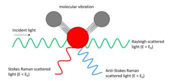
Fig. 1 Raman scattering schematic.
