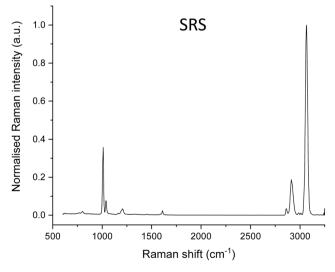
Fig. 5 Uncalibrated spectra obtained from a polystyrene sheet using RS with a range of excitation sources (left), compared to SRS (right). The spectra have been normalised to the highest intensity peak but have not been corrected for wavelength-dependent sensitivity. The SRS spectrum was acquired with 0.2 nm steps of the pump laser wavelength (2 ps pulse width).
