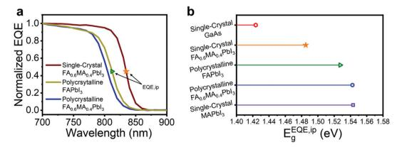
Fig. 4 (a) EQE spectra comparison between the single-crystal  $FA_{0.6}MA_{0.4}PbI_3$  device and polycrystalline  $FAPbI_3$  and  $FA_{0.6}MA_{0.4}PbI_3$  devices with the same device architecture. (b) Bandgap of select absorber materials calculated from the inflection point of the EQE spectrum. The bandgap value for GaAs was obtained from ref. 25.
