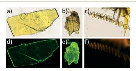
Fig. 4 Optical microscopy images of 4 (a),  $5\alpha$  (b) and  $5\beta$  (c) viewed under visible light and under UV-light emission (4 (d),  $5\alpha$  (e) and  $5\beta$  (f)).
