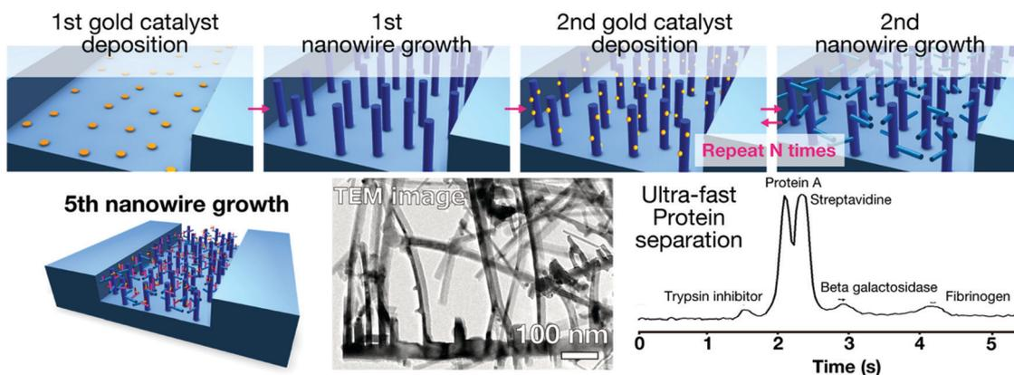
Fig. 7 The 3D nanowire array for ultra-fast separation of biomolecules.<sup>79</sup> The 3D nanowire array was fabricated by repeating catalyst deposition on the targeted special location and nanowire growth from the deposited catalyst.
