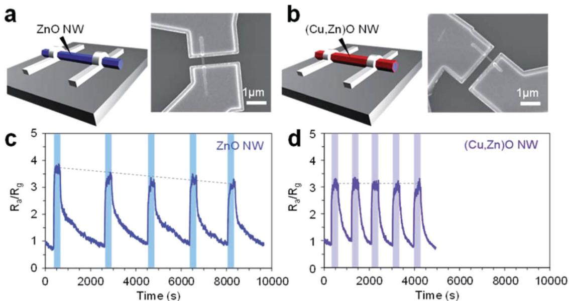
Fig. 9 (a and b) Schematic and SEM images of single nanowire sensor devices using the (a) ZnO nanowire and (b) (Cu,Zn)O nanowire.<sup>99</sup> (c and d) Five successive sensor responses to nonanal using the ZnO nanowire device and (Cu,Zn)O nanowire device, respectively.<sup>99</sup>
