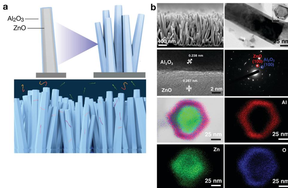
Fig. 3 (a) Annealed ZnO/Al<sub>2</sub>O<sub>3</sub> core/shell nanowires were developed as a platform for capturing RNA molecules.<sup>51</sup> (b) Characterization of the annealed ZnO/Al<sub>2</sub>O<sub>3</sub> core/shell nanowires by scanning electron microscopy (SEM; first row left), transmission electron microscopy (TEM; first row right and second row left), X-ray diffraction (second row right), and TEM-energy dispersive X-ray spectroscopy (third and fourth rows).<sup>51</sup>
