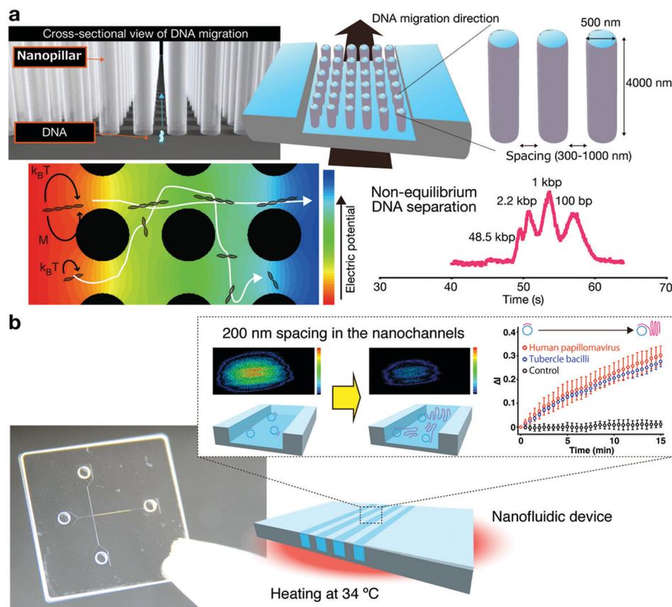
Fig. 6 (a) Non-equilibrium DNA separation using nanopillar arrays.<sup>69</sup> (b) Label-free detection of DNA amplification in a nanofluidic device.<sup>73</sup>
