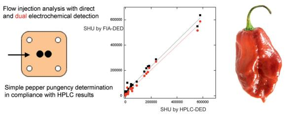
Fig. 1 (A) Schematic image of flow injection analysis with amperometric dual electrode detection using a thin layer cell with glassy carbon working electrodes. The correlation of SHU determined by HPLC-DED and by FIA-DED using E1 (upstream electrode, EDET = 1.0 V; squares) and E2 (downstream electrode,  $E_{DET} = 0.0 \text{ V}$ ; circles) for electrochemical detection is also shown.<sup>39</sup> Reproduced with permission from ref. 39. Copyright Elsevier 2018
