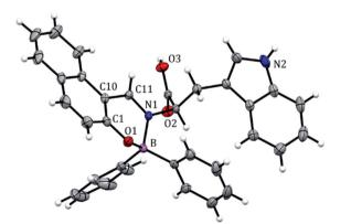
Fig. 1 Crystal structure of BOSCHIBA 3a. Anisotropic displacement parameters are depicted at the 30% probability level. Hydrogen atoms were omitted for clarity. Distances: B(1)-N(1) 1.631, B(1)-O(1) 1.495, B(1)-C(17) 1.614, B(1)-C(23) 1.618, C(11)-N(1) 1.299 Å. Bond angles: C(11)-B(1)-N(1) 118.64, O(1)-B(1)-N(1) 104.22, O(1)-B(1)-C(17)110.89, N(1)-B(1)-C(23) 105.98, C(2)-C(11)-N(1) 122.85, C(11)-N(1)-C(12) 119.38°.
