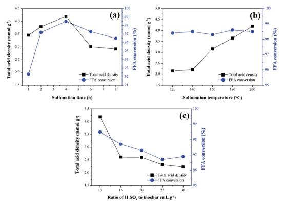
Fig. 2 Influence of sulfonation conditions on the catalytic activity of the sulfonated biochar catalyst (esterification at 90  $^{\circ}$ C for 2 h with the molar ratio of methanol to oleic acid of 20 : 1 and catalyst load of 5 wt%). (a) Sulfonation time (at 200  $^{\circ}$ C and solid-acid ratio of 1 : 10); (b) sulfonation temperature and (at 4 h and solid-acid ratio of 1 : 10); (c) solid-acid ratio of H<sub>2</sub>SO<sub>4</sub> to biochar (at 4 h and 200  $^{\circ}$ C).
