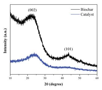
Fig. 3 XRD diffraction patterns of biochar and catalyst.
