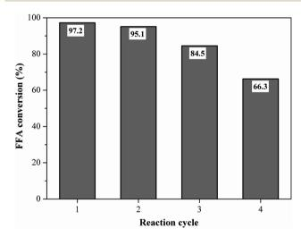
Fig. 11 Reusability study of the catalyst (esterification at  $90 \, ^{\circ}\text{C}$  for  $1.5 \, \text{h}$  with the molar ratio of methanol to oleic acid of 10 : 1 and catalyst load of  $5 \, \text{wt}$ %).
