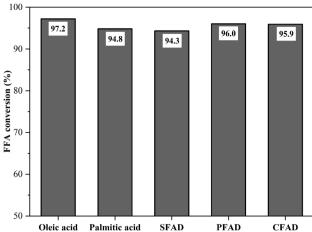
Fig. 10 Catalyst performance on different raw materials (esterification at 90  $^{\circ}$ C for 1.5 h with the molar ratio of methanol to raw material of 10 : 1 and catalyst load of 5 wt%).
